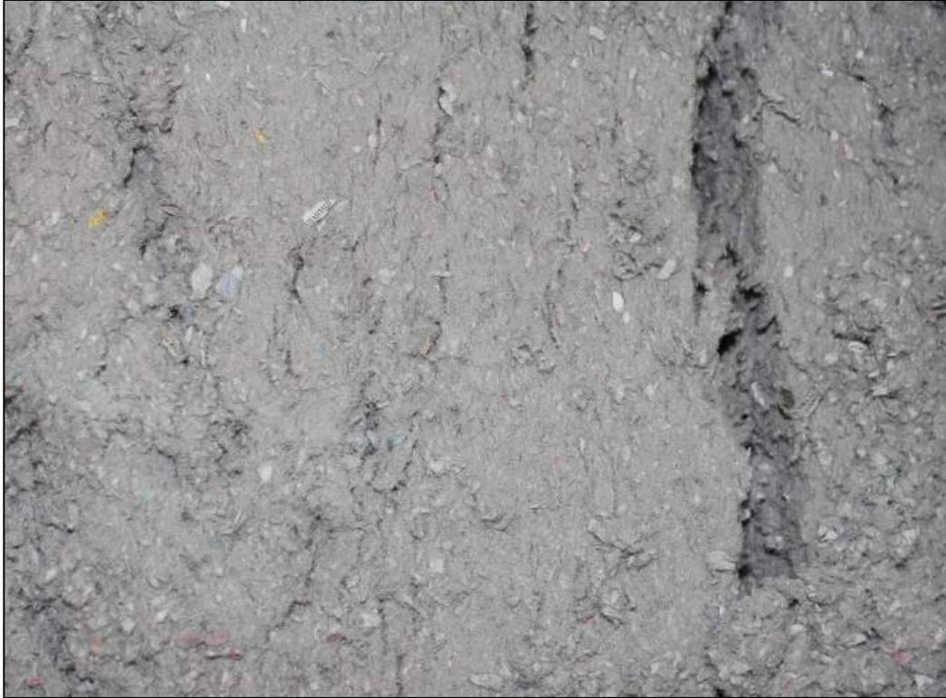
**Figure 4.1: Dry Loose Fill Cellulose Insulation**
