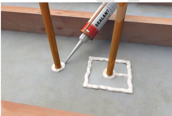
Figure 1: Sealing of Perforations Through Plasterboard Ceiling
